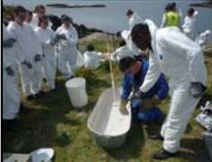
Once the shell had been burnt, the resulting calcium oxide was mixed with cold fresh water resulting in an instantaneous exothermic reaction. This is known as slaking. This image shows the temperature of the slake being taken about 4 minutes after the initial slake. The temp had dropped but was still relatively high 113°C.
